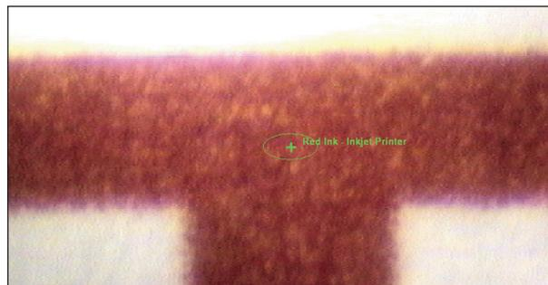
Figure 1: Optical image of one of the samples in the K-Alpha system. The analysis area is defined by the size of the X-ray spot, shown as an ellipse on the image
