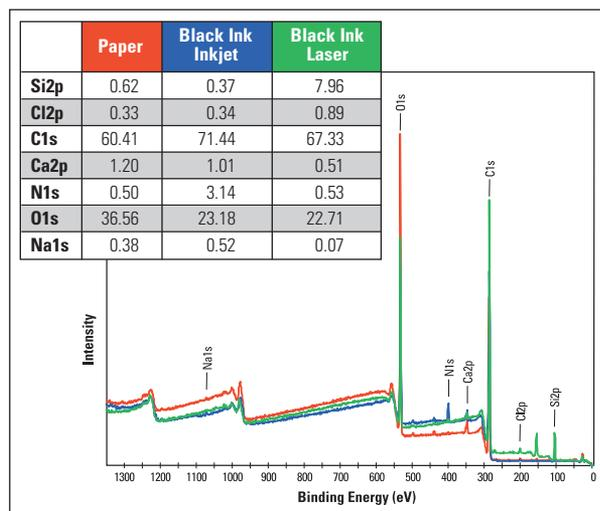
Figure 2: Survey spectra from printed and unprinted areas
