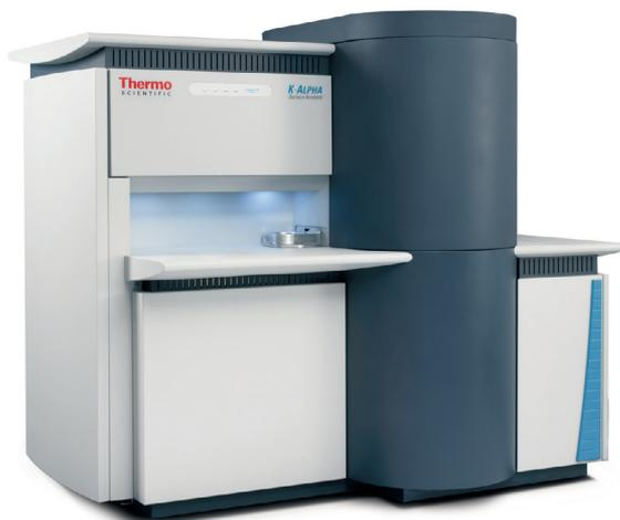
The outstanding XPS sensitivity offered by the K-Alpha system allows for the data to be collected in a very short timeframe without compromising spectral quality. In this case, each survey spectrum took just nine seconds to acquire.
