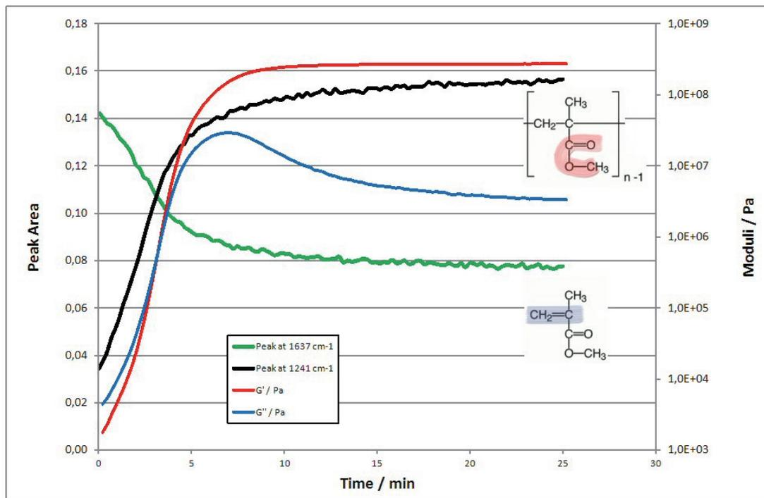
Figure 7: Curing of the acrylate glue monitored with rheology and simultaneous FTIR. The increase of the sample's moduli (red and blue) corresponds with the decreasing signal of the monomer (green) and the increasing signal of the polymer's ester bond (black).
