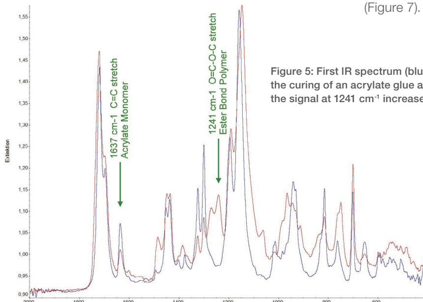
Figure 5: First IR spectrum (blue) and last IR spectrum after 25 min (red) collected during the curing of an acrylate glue at  $23^\circ\text{C}$ . The signal at  $1637\text{ cm}^{-1}$  decreases over time while the signal at  $1241\text{ cm}^{-1}$  increases.
