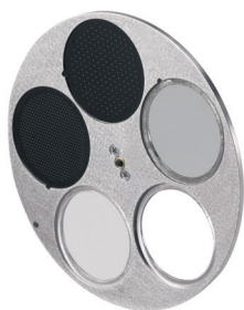
Figure 1: The Nicolet iS20 comes standard with a fully traceable verification wheel
