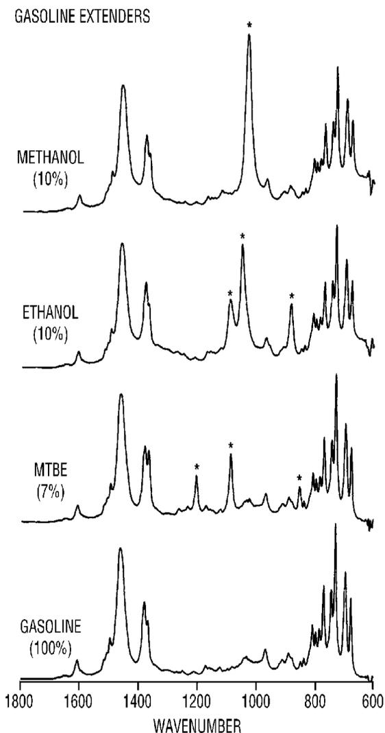
Figure 1: Methanol (10%), Ethanol (10%), and MTBE (7%) in gasoline spectra. Major extender peaks marked with (\*).
