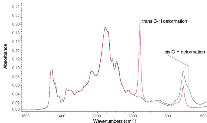
Figure 2: FTIR spectra of *cis* and *trans* fats shows spectral differences distinguishable using FTIR
