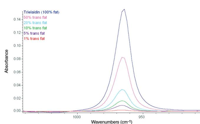
Figure 3: FTIR spectra overlay of trans fat from 1 - 50% with trielaidin (100% *trans*) standard
