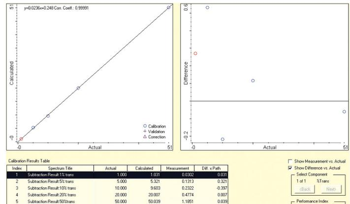
Figure 4: Thermo Scientific TQ Analyst linear regression calibration for *trans* content
