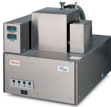
Thermo Fisher Scientific has worked with a major landfill operator to develop a system that can monitor the LFG pre- and post- filter, automatically, every 30 minutes at the landfill site. The Antaris IGS gas analyzer uses FT-IR technology combined with a long path length (2 meter) gas sampling cell to measure total siloxane content using an analytical band at 815 cm<sup>-1</sup> (Figure 3).
