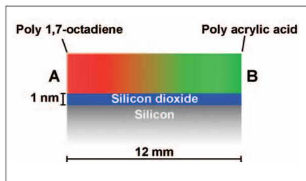
Figure 2: The intended structure of the sample
