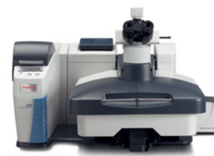
Thermo Scientific DXR Raman microscope or Thermo Scientific Nicolet iN10 microscope For small particle identification or high spatial resolution polymer characterization needs
