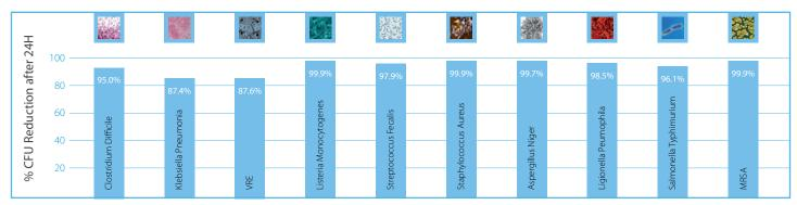
\*In an independent lab test, 10 common microbes were selected, and each of them was incubated on PALOPAQUE HYG panels for 24hrs at 37°C and >90% RH. As the graph shows, HYG panels demonstrate high antimicrobial activity. Use of HYG Products, along with adequate cleaning regime, would significantly reduce microbial growth, including dangerous pathogens.
