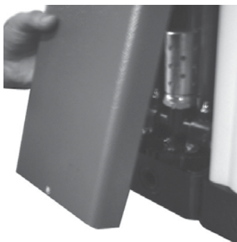
REMOVE FRONT FASCIA PANEL BY TILTING OUTWARDS AND DOWNWARDS.
