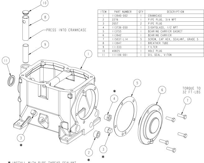
★ INSTALL WITH PIPE THREAD SEALANT
